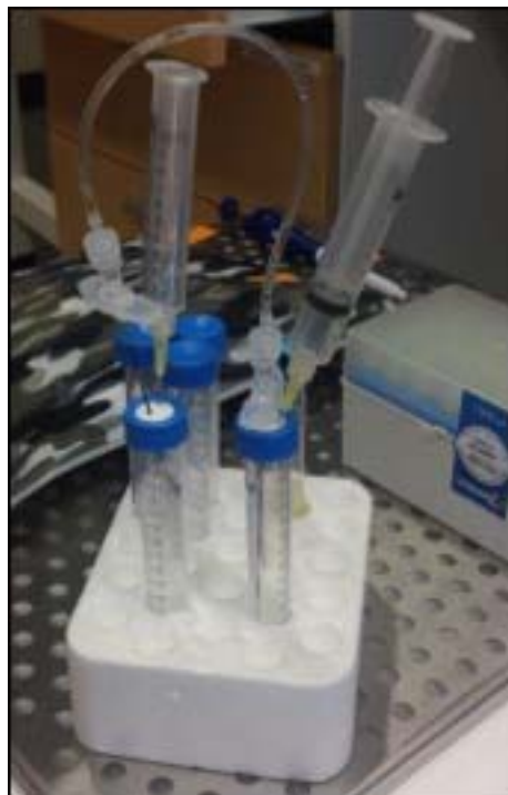
Supplemental Figure 1. Terrestrial set up of cannula transfer. Tygon tubing attached to two needles connects two 15 ml conical tubes with and without liquid. A syringe is used to inject air into the liquid containing tube to force the liquid through the tubing into the empty tube. A syringe without a plunger is used to vent the displaced air from the empty tube as liquid enters.
