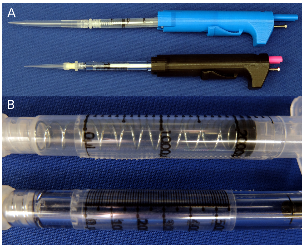
Figure 3: Photos of assembled pipettes. (A) Two assemblies of the pipette: the 100-1000 \mu\text{L} configuration (above) and the 30-300 \mu\text{L} configuration (below). (B) Close-up photo of the taped on scale for each of the syringes.
