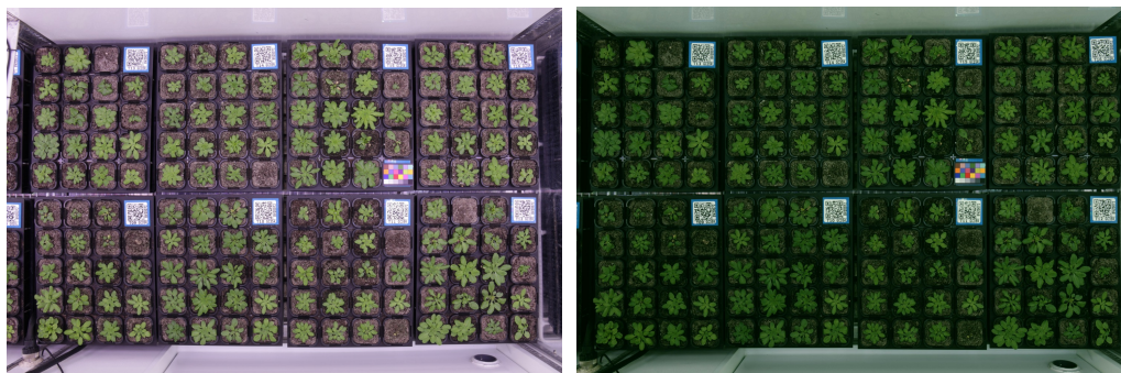
Figure 6: Growth chamber. Left: The original picture of a growth chamber; Right: The result of camera distortion removal and color correction step.
