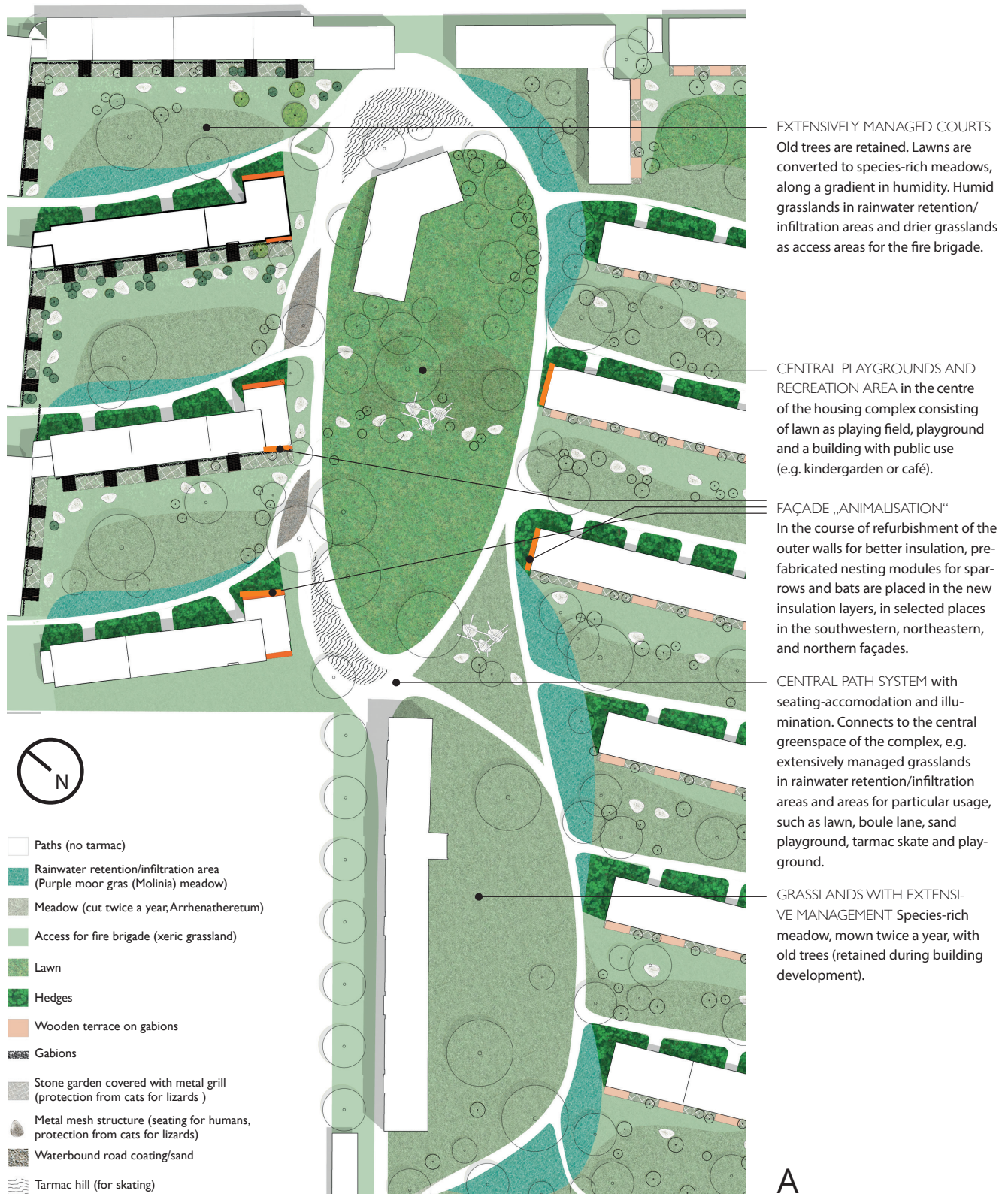
Figure 6: Application of AAD to the refurbishment of an apartment block from the 1960s in Munich, Germany. Such residential areas consisting of several apartment blocks with rental flats were built after the Second World War all over Germany and are now in need of refurbishment including the green space around them. The aim in this theoretical (i.e. not realized) study was to refurbish the building face with increased insulation as an adaptation to climate change, to increase the attractiveness of the greenspace, and to use the public and semi-public space as contribution for the green
